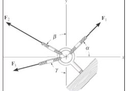
Given:  $F_1 = 600 \text{ N}$   $F_2 = 800 \text{ N}$   $F_3 = 450 \text{ N}$  $\alpha = 45 \text{ deg m } \beta = 60 \text{ deg}$   $\gamma = 75 \text{ deg}$
