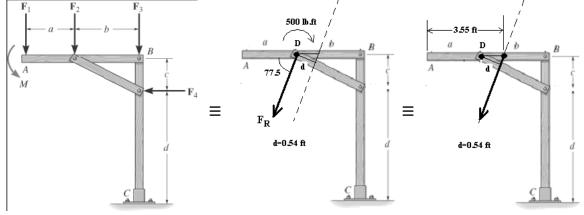
*Given:* M = 600 lb ft *F*<sub>1</sub> = 300 lb, *F*<sub>2</sub> = 200 lb, *F*<sub>3</sub> = 400 lb, *F*<sub>4</sub> = 200 lb a = 3 ft, b = 4 ft, c = 2 ft, d = 7 ft *Solution: F*<sub>Rx</sub> = -*F*<sub>4</sub> *F*<sub>Ry</sub> = -*F*<sub>1</sub> - *F*<sub>2</sub> - *F*<sub>3</sub> *F*<sub>Ry</sub> = -900 lb *F* =  $\sqrt{F_{Rx}^2 + F_{Ry}^2}$  *F*<sub>R</sub> = 922 lb  $\theta = \operatorname{atan}\left(\frac{F_{Ry}}{F_{Rx}}\right)$  $\theta = 77.5 \text{ deg}$
