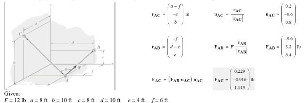
Determine the projected component of the force  $\mathbf{F}$  acting along the axis AB of the pipe.
